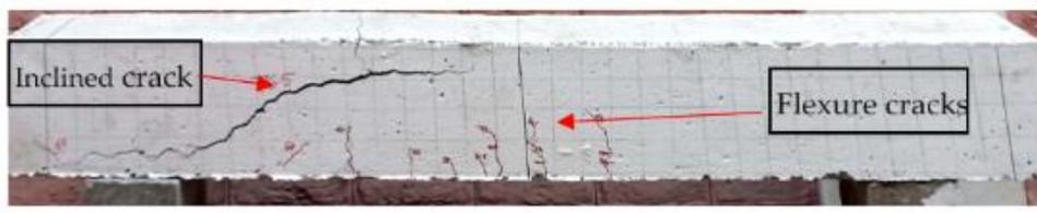
Figure 3. Failure mode of Beam ON-4.5.
