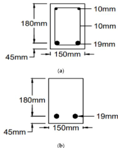
**Figure 1.** (a) Cross-sectional details of beams (a) with shear reinforcement and (b) without shear reinforcement, and longitudinal sectional details of beams
