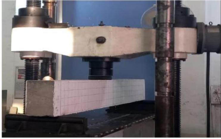
Figure 2. Test set up for three-point bending test.
